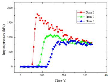
**Impact force** exerted by the debris flow on the check dams are investigated using the **flow-structure coupled SPH method**, the check dams effectively prevented further propagation of debris flow.
