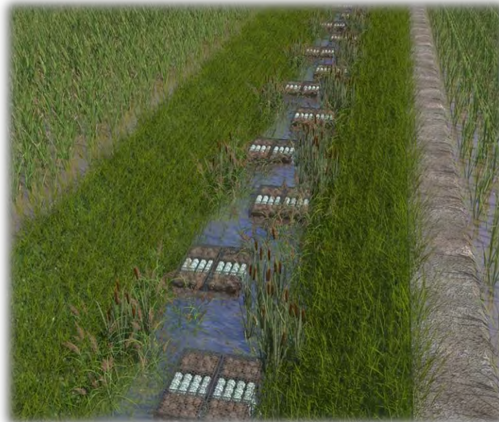
Water purification device for the first stage of farmland back water ZL 201410215464.4
